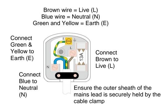
If colours of the wires in the mains lead of this appliance do not correspond with the coloured marking identifying the terminals in your plug, proceed as follows:
