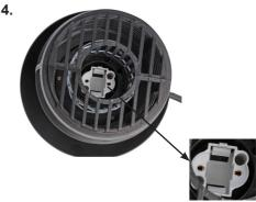
When inserting the new lamp make sure the pins on the lamp, line up with the holes in the lamp holder (see above) inside the appliance and it is fitted securely.
